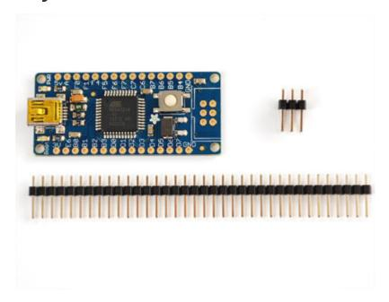
The breakout is almost completely assembled. We don't solder on the header or 6-pin ISP connector since we find it's easy to do but hard to undo, in case you want to put different headers on, or just connect up wires directly.
