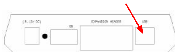
Figure 5. ADC08(B)3000RB rear panel showing location of USB connector
