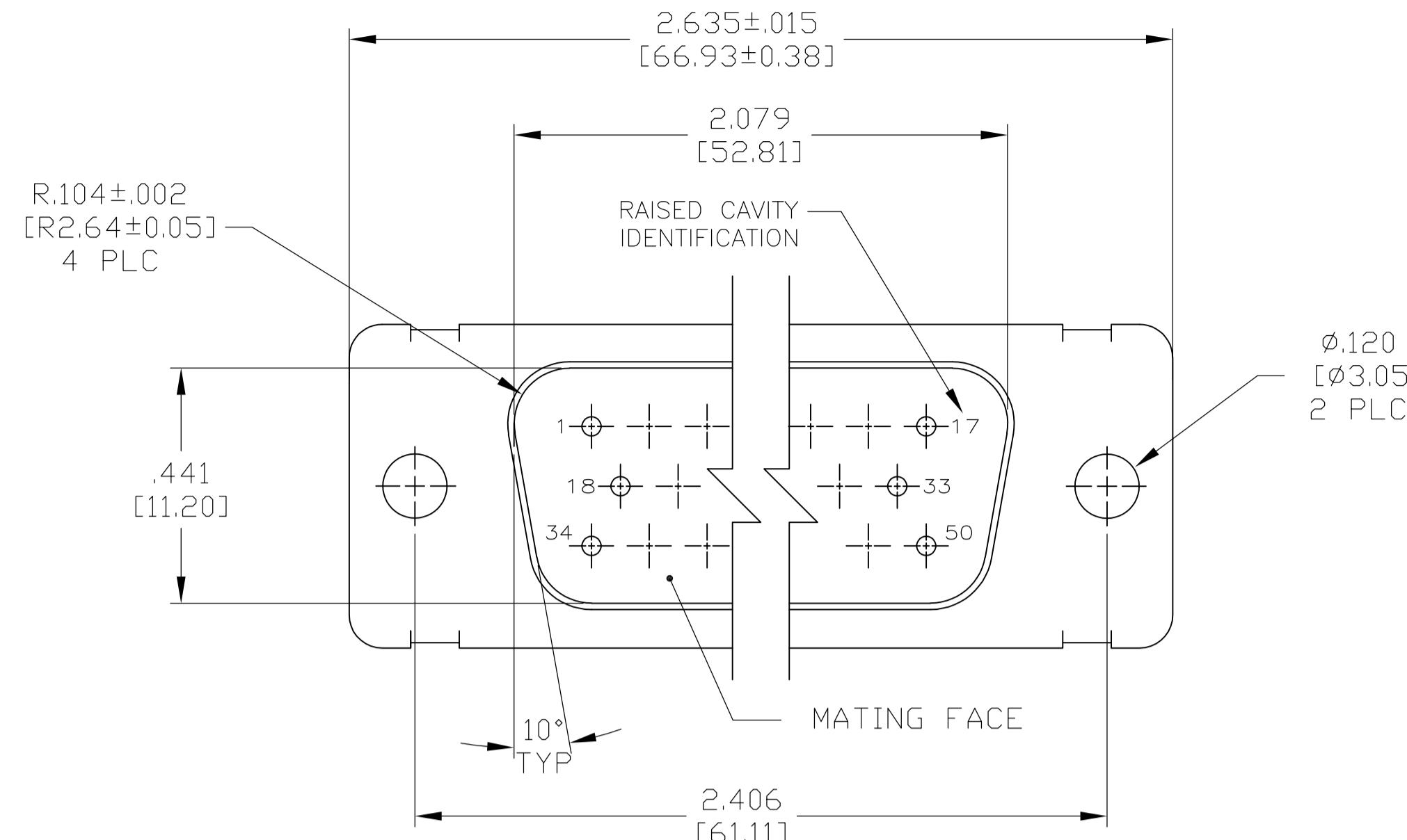
1. THIS CONNECTOR ASSEMBLY IS SUPPLIED WITH Be Cu CONTACT RETENTION CLIPS INSTALLED IN THE INSERT ASSEMBLY.
