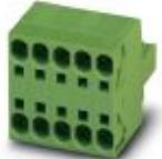
PCB connector, nominal current: 41 A, rated voltage (III/2): 1000 V, nominal cross section: 6 mm<sup>2</sup>, number of positions: 9, pitch: 7.62 mm, connection method: Push-in spring connection, color: green, contact surface: Tin
