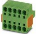
PCB connector, nominal current: 41 A, rated voltage (III/2): 1000 V, nominal cross section: 6 mm<sup>2</sup>, number of positions: 9, pitch: 7.62 mm, connection method: Push-in spring connection, color: green, contact surface: Tin
