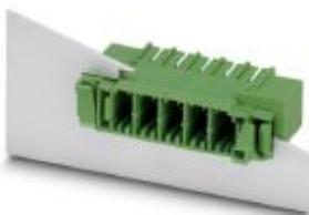
Feed-through header, nominal current: 41 A, rated voltage (III/2): 630 V, nominal cross section: 6 mm<sup>2</sup>, number of positions: 9, pitch: 7.62 mm, color: green, contact surface: Tin, mounting: Wave soldering, pin layout: Linear pinning, solder pin [P]: 4.9 mm
