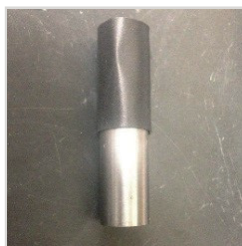
CORRECT ID PLUG GAGE KEEPS TUBING ROUND
