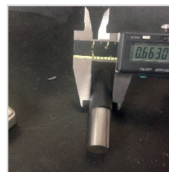
CORRECT OD PLUG GAGE KEEPS TUBING FROM BEING SQUEEZED
