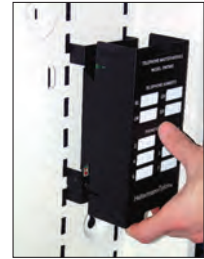
Step 3 - Push cover on module
