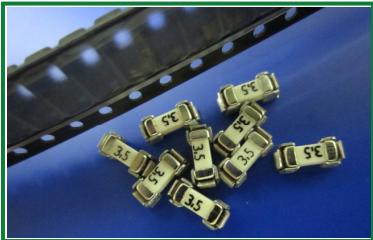
These fuse/clip assemblies can be efficiently placed in a single pass. Once reflowed, fuse replacement requires no resoldering.
