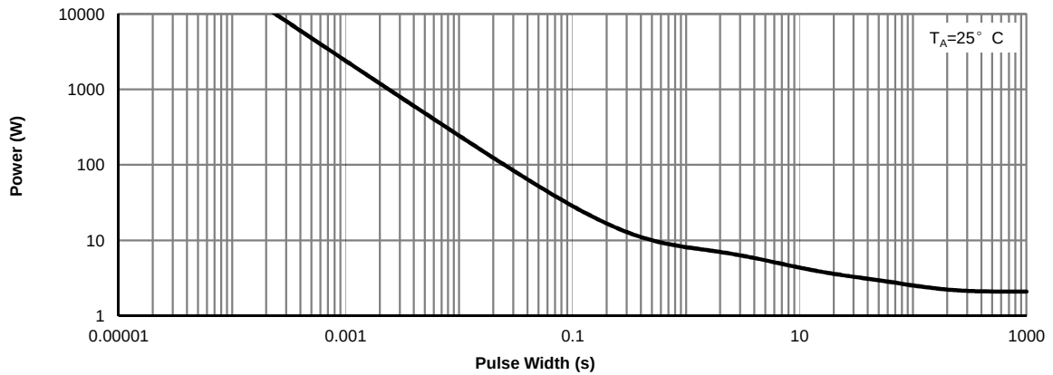
Figure 14: Single Pulse Power Rating Junction-to-Ambient (Note H)
