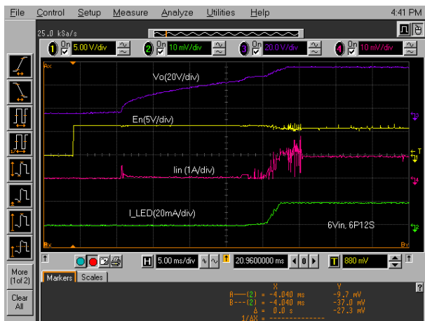
FIGURE 12. IN-RUSH AND LED CURRENT AT V_{IN} = 6V FOR 4P12S AT 20mA/CHANNEL
