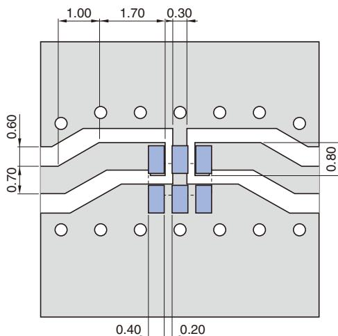
Line width be designed to match  $50\Omega$  characteristic impedance depending on PCB material and thickness.
