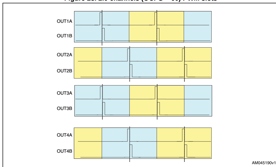
Figure 28. 2.0 channels (OCFG = 00) PWM slots
