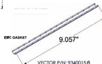
VECTOR P/N: 93400156 MATERIAL: STEEL WITH BRIGHT NICKEL FINISH
