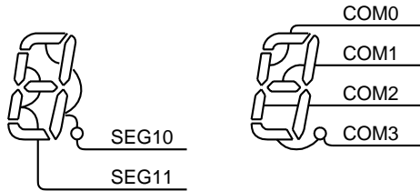
Figure 15-5 Example of COM, SEG Pin Connection (1/4 duty)
