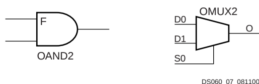
Figure 7: AND and MUX Symbols in Spartan-XL IOB
