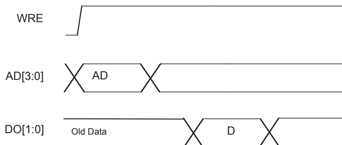
Figure 3-7. Slice Single /Dual Port Read Cycle Timing
