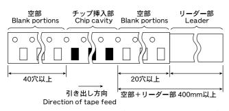
Insertion leader is 400 mm or more (including 20 empty cavities) Empty cavities at end of reel: 40 holes or more
