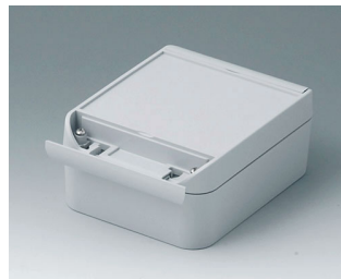
C6011141 SMART-BOX WIDTH 4.331" ASA+PC-FR (UL 94 V-0) light gray RAL 7035 5.51"x4.33"x2.36" IP 66
