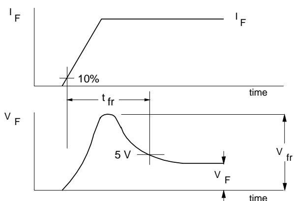
Fig. 3. Definition of anti-parallel diode  $V_{fr}$  and  $t_{fr}$ .
