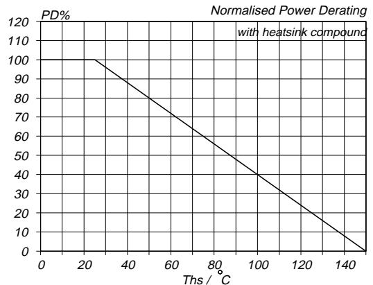
Fig.10. Normalised power dissipation.
