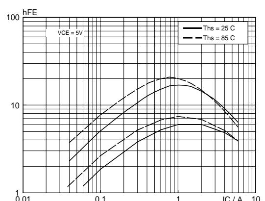
Fig. 6. High and low DC current gain.
