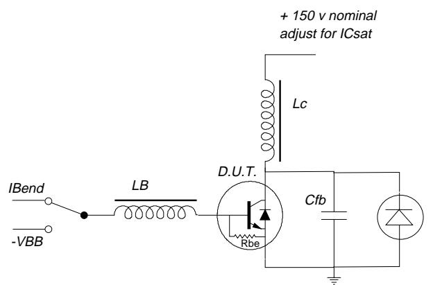
Fig. 4. Switching times test circuit.
