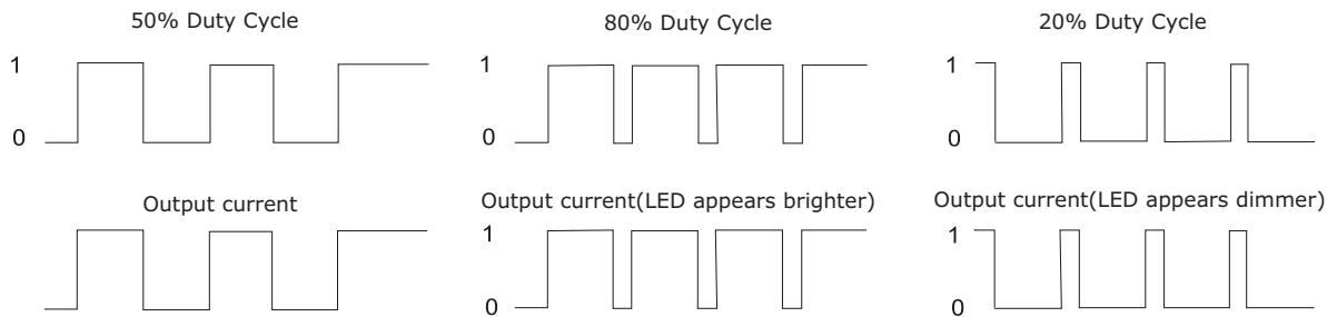
For the rated frequency PWM dimming, the output current of driver matters to the pulse width of the PWM signal, and the numerate please refer to the following formula:
