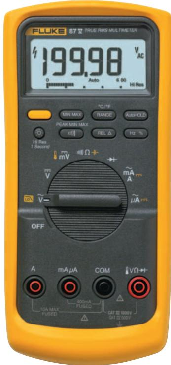
The new Fluke 87V has improved measurement functions, troubleshooting features, resolution and accuracy to solve more problems on motor drives, in plant automation, power distribution, and electro-mechanical equipment. The 87V operates very similar to the classic 87, but with more problem-solving power, safety, convenience and impact protection.
