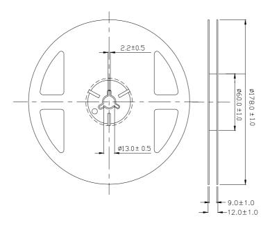
**Note:** The tolerances unless mentioned is  $\pm 0.1$ mm ,Unit = m
