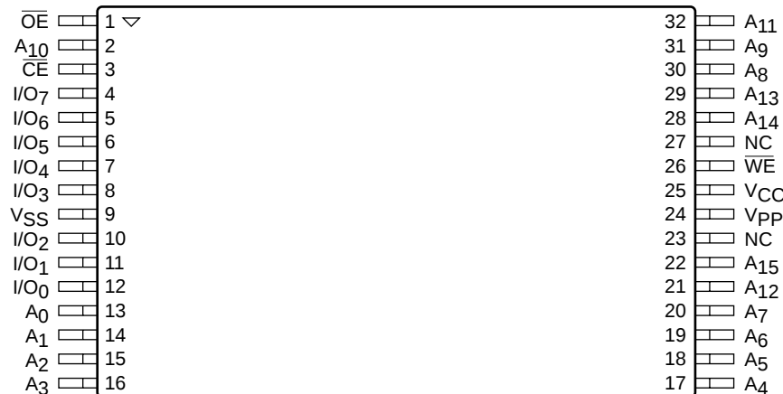
TSOP Package (Reverse Pinout) (TR, HR)
