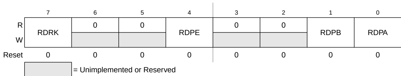
Figure 18-15. Reduced Drive Register (RDRIV)
