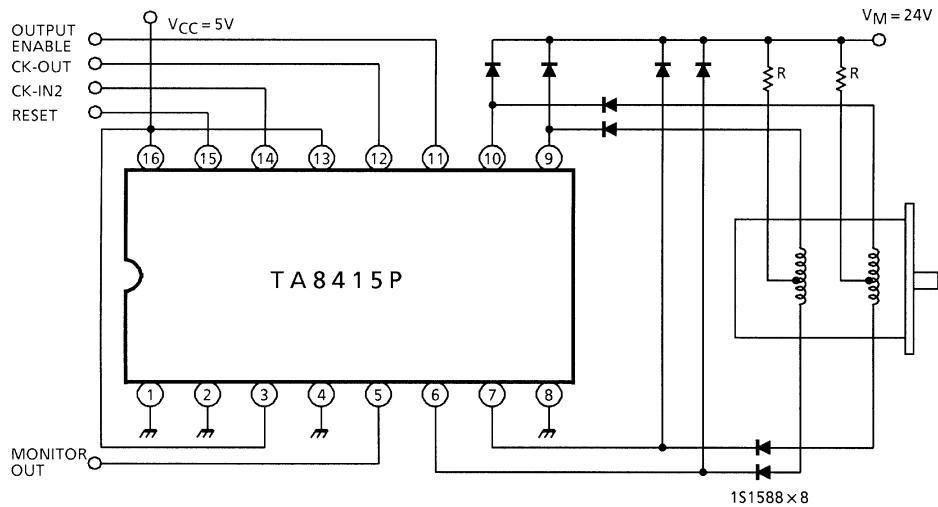
Note: Utmost care is necessary in the design of the output line, power supply and GND line since IC may be destroyed due to short-circuit between outputs, air contamination fault, or fault by improper grounding.
