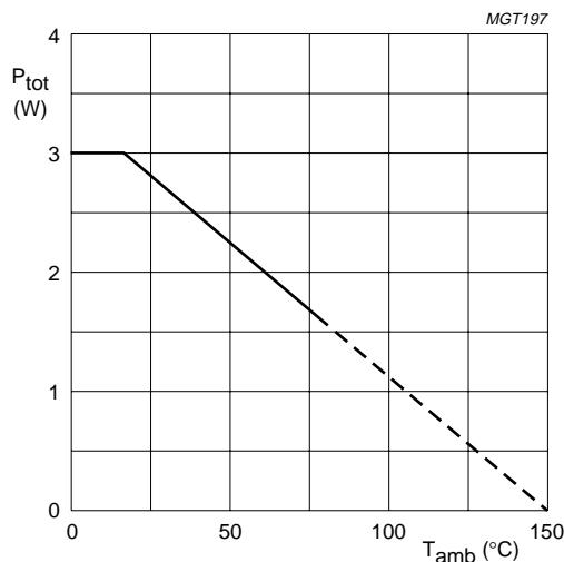
The IC is thermally connected with its heatsink to an external heatsink at ambient temperature, with a total thermal resistance of 35 K/W (10 K/W junction to case plus 25 K/W case to surrounding).
