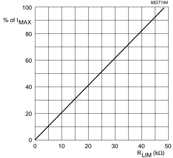
Fig.7 Maximum output current as a function of  $R_{LIM}$ .
