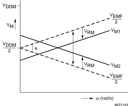
Fig.6 Motor voltage when actively braking.
