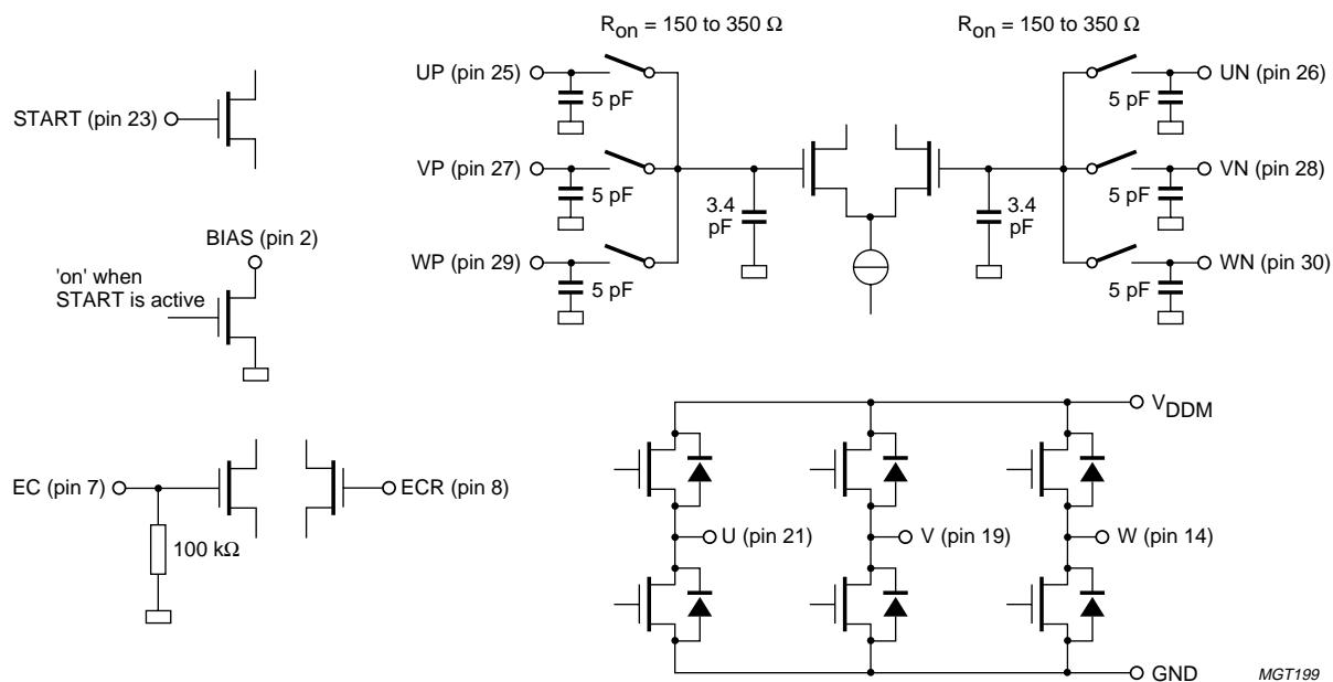
Fig.11 Input and output equivalent circuits.
