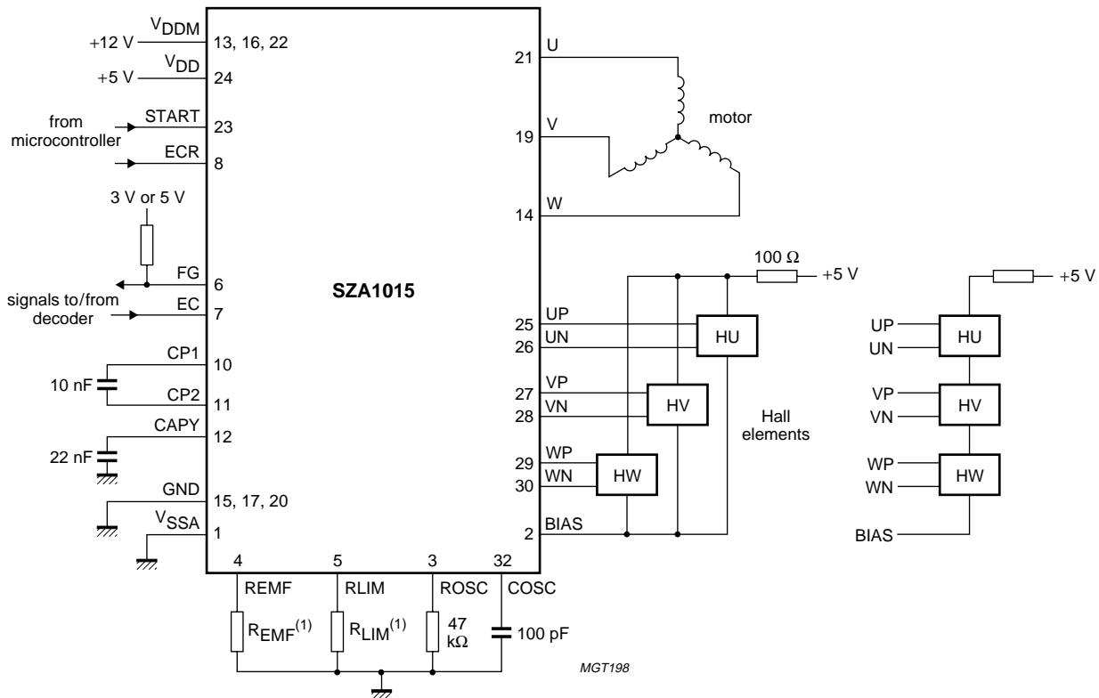
(1) For selection of the resistors  $R_{EMF}$  and  $R_{LIM}$  see Chapter "Functional description".
