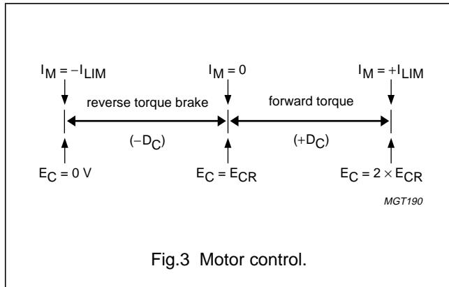
The gain from input voltage ( $E_C$ ) to motor current ( $I_M$ ) is  $I_{LIM}/E_{CR}$  (A/V). The motor current can be determined with the following formula:  $I_M = \frac{I_{LIM}}{E_{CR}} \times (E_C - E_{CR})$
