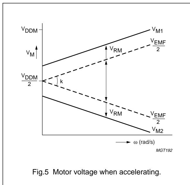
If we assume that  $I_{MACC}$  is used to accelerate and  $I_{MBR}$  is used to brake we can draw two pictures shown in Figs 5 (accelerate) and 6 (brake).
