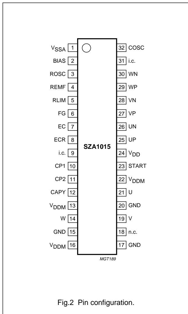
Fig.2 Pin configuration.
