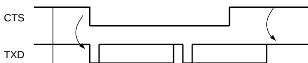
Figure 20-16. Transmitter Behavior when Operating with Hardware Handshaking
