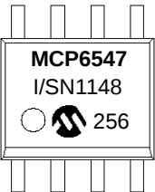
8-Lead SOIC (150 mil) (MCP6546, MCP6547, MCP6548, MCP6549)
