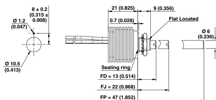
Available only with bushing M10 x 0.75 and shafts Ø 6 mm
