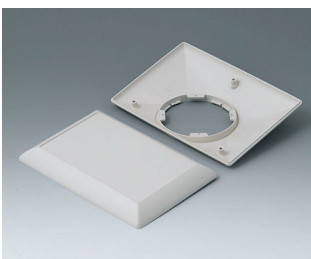
B5017207 Bottom and top part E160 F ABS (UL 94 HB) off-white RAL 9002 6.30"x4.33"x1.50"
