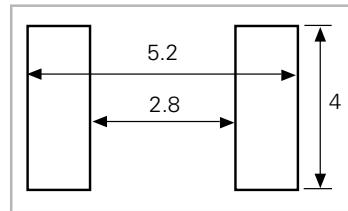
Recommended Soldering Pad Layout
