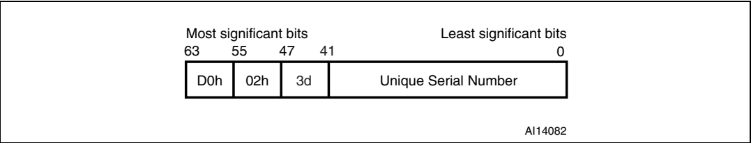
Figure 50. 64-bit unique identifier of the SRIX4K
