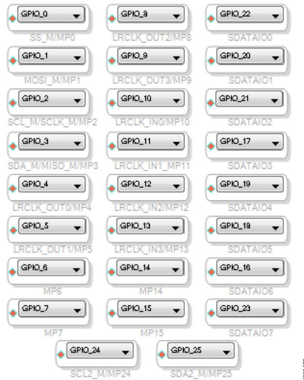
Figure 79. Complete Set of General-Purpose Outputs in SigmaStudio
