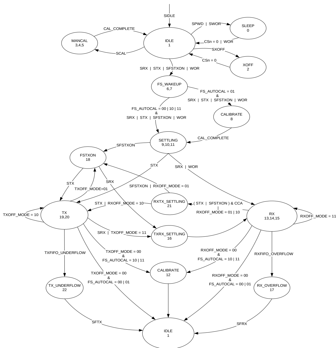
Figure 25: Complete Radio Control State Diagram
