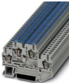
Double-level spring-cage terminal block, connection method: Spring-cage connection, cross section: 0.08 mm 2 - 4 mm 2 , AWG: 28 - 12, width: 5.2 mm, color: gray, mounting type: NS 35/7,5, NS 35/15
