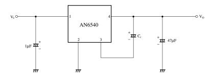
$\bullet$  Choose the oscillation control capacitor 47 $\mu$ F which has a small capacitance reduction even at a low temperature. For example, use the tantalum capacitor.
