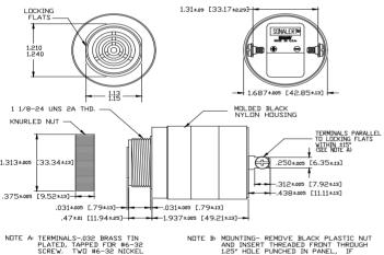
NOTE B: MOUNTING- REMOVE BLACK PLASTIC NUT AND INSERT THREADED FRONT THROUGH 125' HOLE PUNCHED IN PANEL, IF DRIENTATION IS NEEDED, NOTE LOCKING FLATS ON DRAWING. SCREW NUT BACK ON. DO NOT DVERTIGHTEN.
