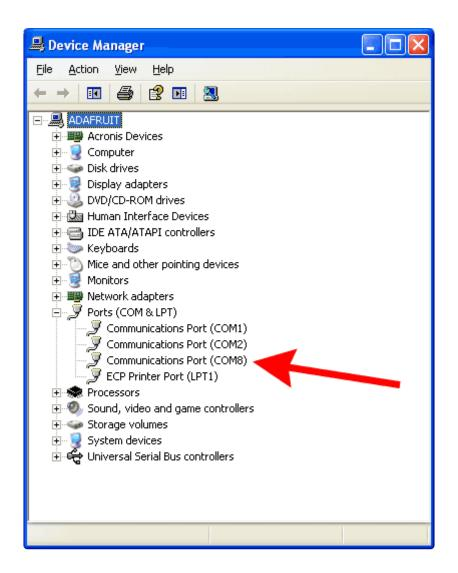
For mac/linux, once you have plugged in the cable, run **dmesg** to see what the name of the port is, probably something like /dev/cu.usbmodem-XXXX or similar. You can also type **Is** /dev/cu.\* into a **Termnal** window and see what items appear/disappear when the cable is connected and unplugged.
