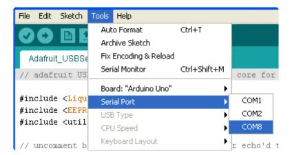
Open the serial port monitor and type Hello World! into the text box.
