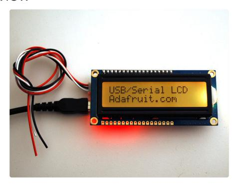
Adding a character display to your project or computer has never been easier with the new Adafruit USB or TTL serial backpack! This custom-designed PCB sits on the back of <u>any 'standard' character LCD (16x2 or 20x4 sized)</u> (https://adafru.it/alS) and does everything you could want: printing text, automatic scrolling, setting the backlight, adjusting contrast, making custom characters, turning on and off the cursor, etc.
