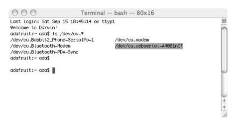
Now that the port is known, you can use your favorite terminal program to connect. For this example, we'll use the basic terminal built into Arduino. The only downside of the serial port monitor is that you can only send a full string at a time and there's a
