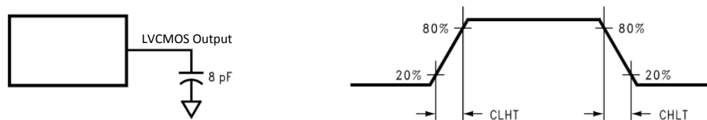
Figure 2. LVCMOS Output Load and Transition Times
