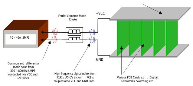
With a broad band ferrite common mode choke in place the effects of a high current are negated and thus saturation of the choke is not an issue.
