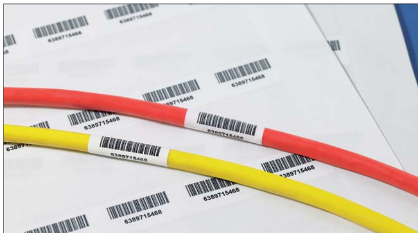
Laminating the mark gives long-term print survivability.
