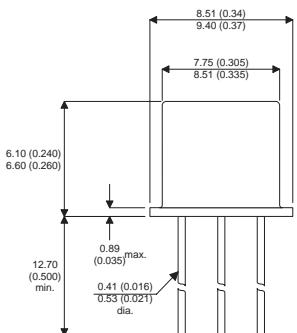
**Bipolar NPN Device in a
