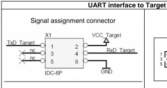
View onto wiring pin configuration
