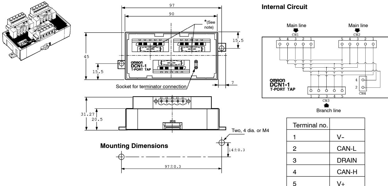
**Note:** When connecting a branch line to the main line, connect the main line to the connector marked with an asterisk because the resistance between the asterisked portion is minimal.
