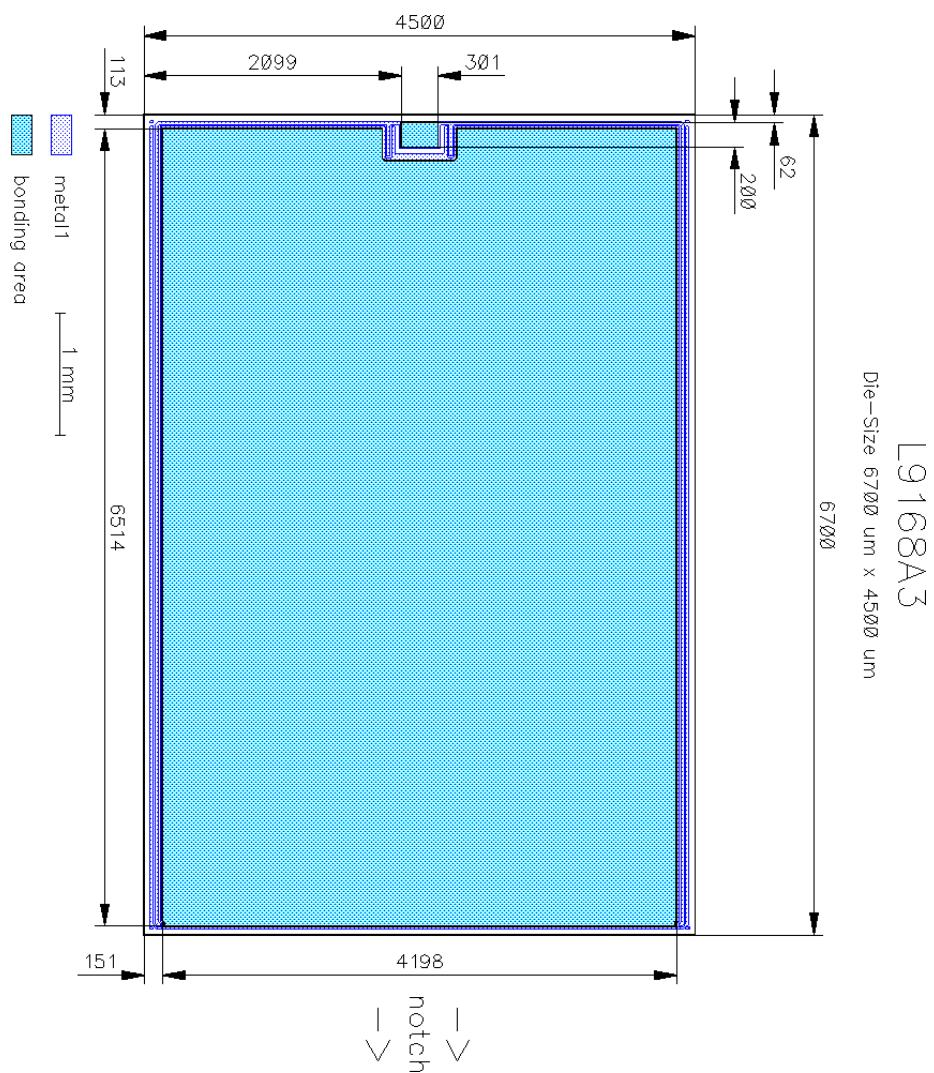
**Figure 1 Outline Chip, dimensions in μm**
