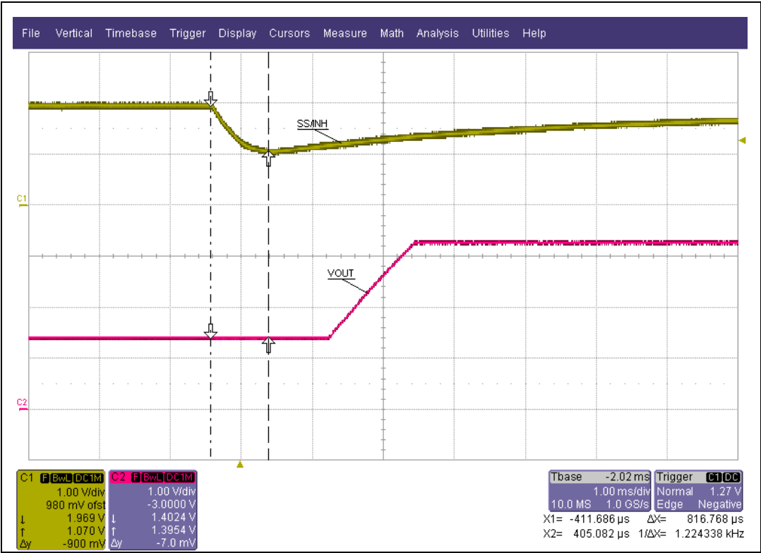
Figure 9. External soft-start after UVLO or thermal shutdown
