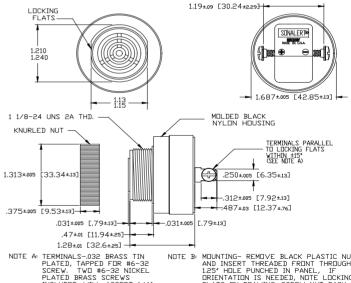
NOTE A: TERMINALS-0.02 BRASS IIN PLATED, TAPPED FOR #6-32 SCREW. TWU #6-32 NICKEL PLATED BRASS SCREWS INCLUBED. WILL ACCEPT 1/4\* QUICK CONNECT.
