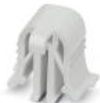
Switching lock, for additional locking of short-circuit switching elements in current transformer measuring circuits, Length: 16.3 mm, Width: 12.5 mm, Height: 13.6 mm, Color: white
