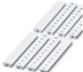
Zack marker strip, Strip, white, labeled, can be labeled with: Plotter, Printed horizontally: Consecutive numbers 1 - 10, 11 - 20, etc. up to 491 - 500, Mounting type: Snap into tall marker groove, for terminal block width: 8.2 mm, Lettering field: 10.5 x 8.15 mm
