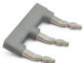
Insertion bridge, Pitch: 16.4 mm, Length: 24 mm, Width: 39 mm, Number of positions: 3, Pin assignment: 1,3,5, Color: gray
