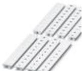
Zack marker strip, Strip, white, labeled, can be labeled with: Plotter, Printed vertically: Consecutive numbers 1 - 10, 11 - 20, etc. up to 91 - 100, Mounting type: Snap into tall marker groove, for terminal block width: 8.2 mm, Lettering field: 10.5 x 8.15 mm
