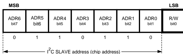
Figure 8. I 2 C Chip Address
