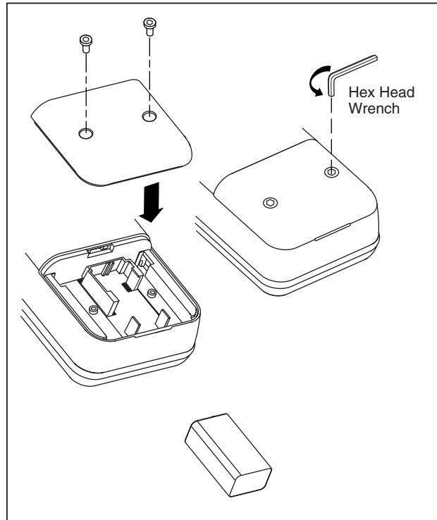
Figure 7. Battery Replacement
