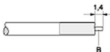
C Push contact (1) onto cable inner conductor up to the cable dielectric and crimp on with square 0.75 A/F.
