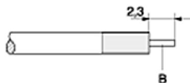
C Insert cable into body (1). Solder cable jacket and body all around.
